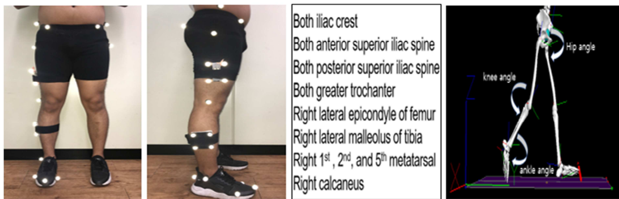
Figure 2. Reflective marker position (left and middle) & definition of joint coordinate system (right)
